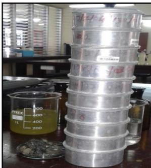
Plate 1: Mud sample analysis by using sieve set
