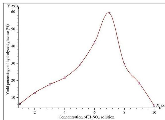
Figure 3: The yield percentage of hydrolyzed glucose from  $1.0 \times 10^4$  ppm of extracted cellulose with the constant agitating speed (400 rpm) for 4 hours and maintained at  $30^\circ\text{C}$  for the various concentration of  $\text{H}_2\text{SO}_4$  solution.
