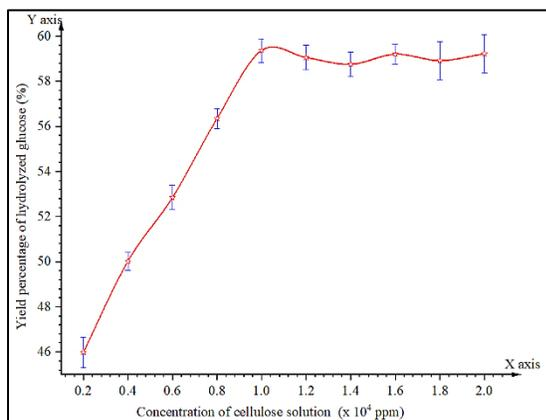
Figure 2: The yield percentage of hydrolyzed glucose as a function of extracted cellulose from PFH fibers with a constant agitating speed (400 rpm) and concentration of  $\text{H}_2\text{SO}_4$  ( $7.0 \text{ mol L}^{-1}$ ) for 4 hours at  $30^\circ\text{C}$ .
