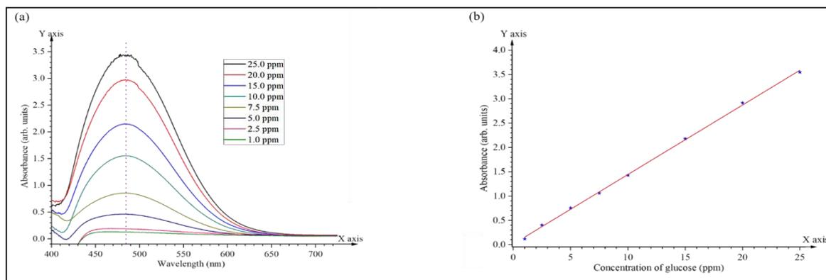
Figure 1: (a) The absorbance spectra of various concentration of standard glucose solutions in the presence of DNS reagent within the wavelength range 400 nm – 720 nm and (b) The standard calibration curve for the standard glucose solution at the optimum wavelength 484.0 nm.
