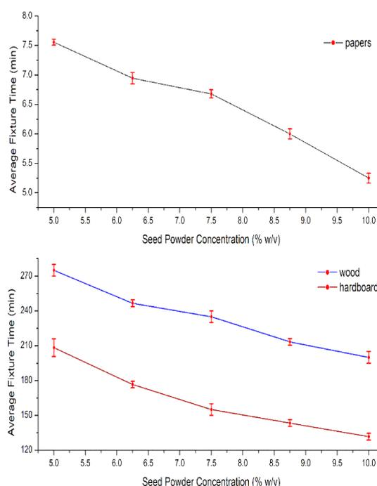
**Figure 2: Fixture time variation with respect to seed powder concentration for different materials**
