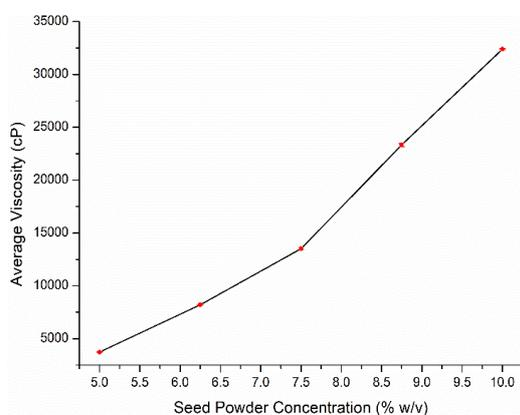
**Figure 1: Viscosity of the glue samples Vs the seed powder concentration**
